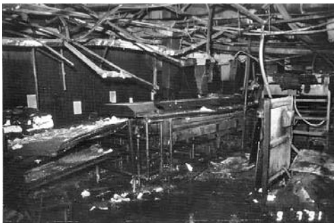
Two views of cooker vat where fire started in chicken processing plant in Hamlet, N.C., in 1991, killing 25 workers.
