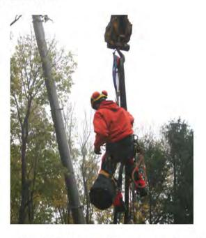
ACCEPTABLE: Climbing line run through master link. Crane hook is latched and wired shut. Various size slings remain in the hook.
