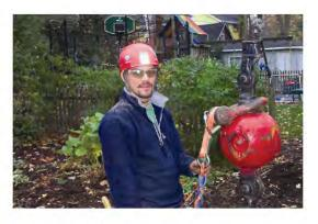
ACCEPTABLE: Locking carabiner simultaneously captures the friction-saver and "locks" the shackle pin.
