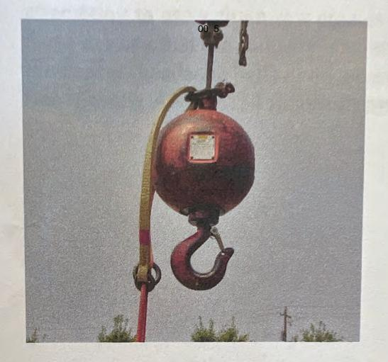
ACCEPTABLE: shackle above the ball, pin wired in place, climbing line in friction-saver.
