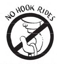
UNACCEPTABLE: Climbers must avoid placing climbing line or lanyard directly into the hook and certainly not in a hook that isn't latched and "locked".
